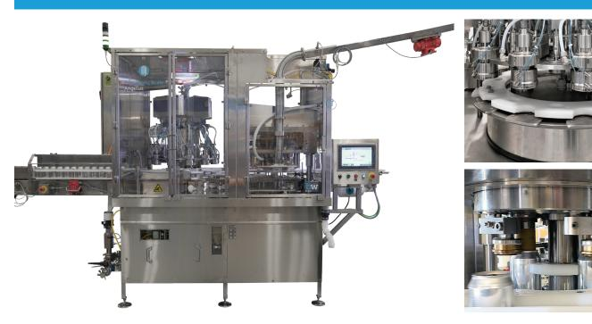
The CB100R counter-pressure canning line employs a 12-head rotary filling turret, coupled with a 3-spindle rotary seamer, to allow the machine to fill more than 100 CPM. The full rotary, continuous motion design ensures the smooth transition of cans through the system at higher speeds, effectively limiting agitation that can reduce product quality.
