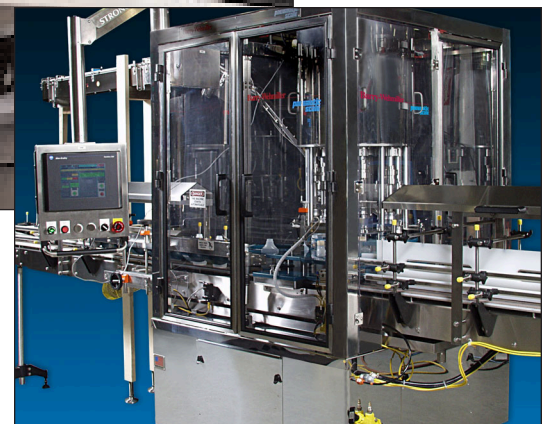
The TC Capper, shown with optional mirror-finish stainless steel, is available as a free-standing turret and in stand-alone or monoblocked configurations.
